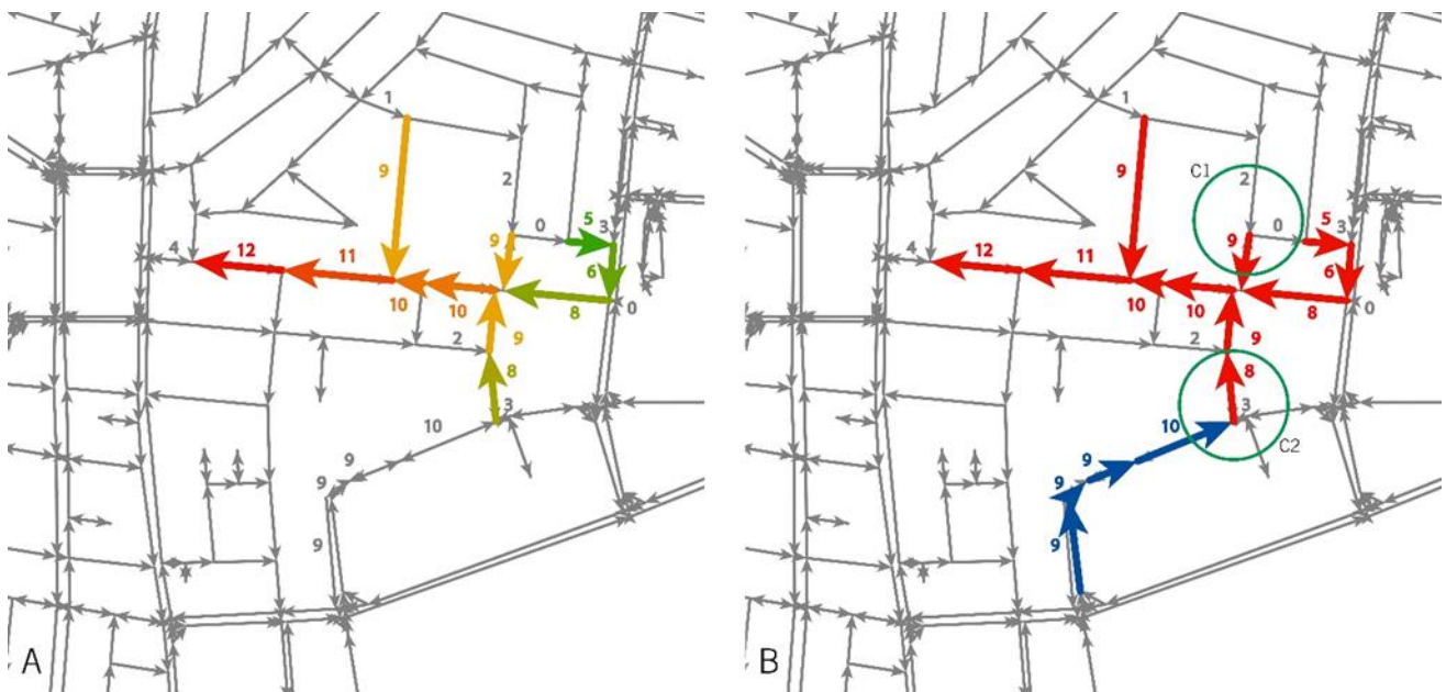
Figure 1: Clusters of JTs. (A) All the colored streets are part of one JT (B) Two JTs (represented by red and blue colors). The red JT does not include the street that has been loaded for 2 measurements, as the time gap between this street and its adjacent one is larger than the pre-defined threshold (see the upper green circle). The blue JT cannot be considered as part of the red JT, as the duration of its trunk is longer than that of its adjacent street in the red JT (see the lower green circle).
