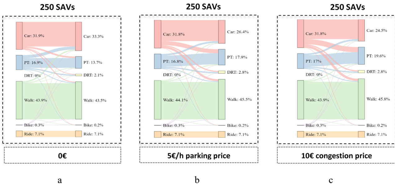
Figure 5: Sankey diagrams of modal split change only for the city center with 250 SAVs ( core-periphery SAV service ); (a) 250 SAVs, 0€; (b) 250 SAVs, 5€/h parking price and (c) 250 SAVs, 10€ congestion price.
